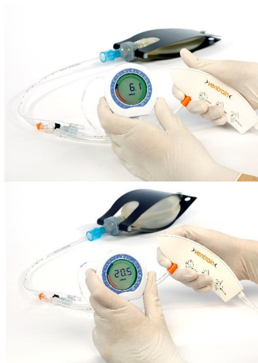
Fig. (8). Illustration of the Tritube® used in conjunction with the Ventrain® and attached to a test lung. A manometer connected to the Tritube®'s pressure measurement lumen enables continuous monitoring of intratracheal pressures. In this arrangement the test lung pressure ranges from a minimum of 6.1 cm H 2 O (PEEP) (top image) to a peak inspiratory pressure of 20.5 cm H 2 O (bottom image).
